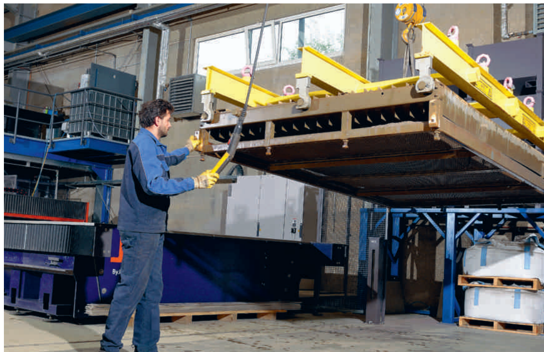
Top: Cleaning the ByJet Pro L. Center: Operation of the machine is simple and highly intuitive. Bottom: The exchangeable cassettes, together with lifting equipment, allow easy unloading of parts.
