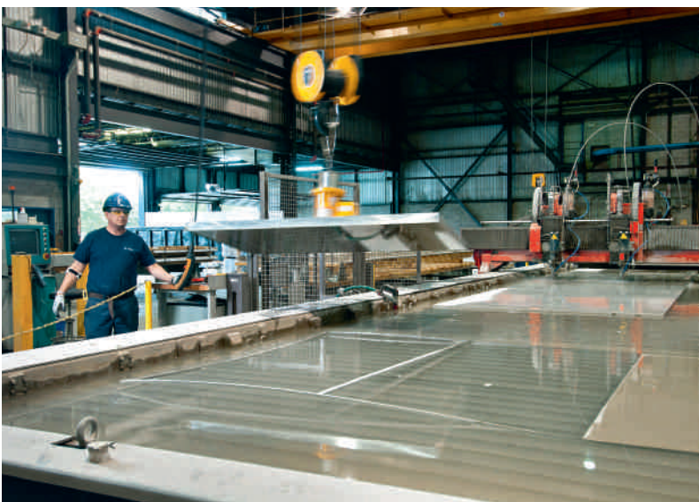
The Byjet L 10030 can process large parts of up to ten meters long and three meters wide. It can also be operated like a shuttle table system.
